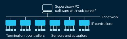
\*Supervisory BMS software with web server is not typically run on a fan-less embedded platform or on a server in the IT suite rather than on a desktop PC
